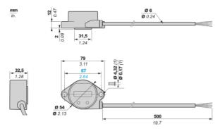
(1): The sensor is supplied with 2 stainless steel inserts and 2 silicone washers. M4 screws not provided.
