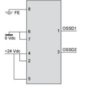
With External Device Monitoring (EDM) feedback loop
