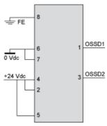
With External Device Monitoring (EDM) feedback loop
