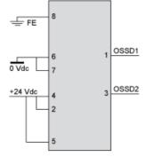
With External Device Monitoring (EDM) feedback loop
