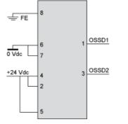
With External Device Monitoring (EDM) feedback loop
