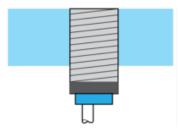
Fixing nut tightening torque: 40 N.m
