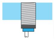
Fixing nut tightening torque: 40 N.m
