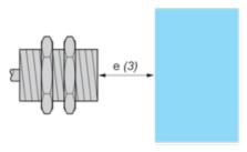
e (3) ≥ 30 mm/1.18 in Mounted in a metal support
