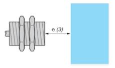
e (3) ≥ 12 mm/0.47 in. Mounted in a metal support
