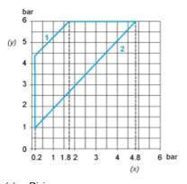
(y) Rising pressure(x) Falling pressure1: Maximum differential
