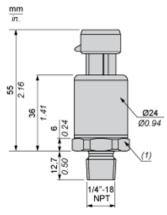
(1) SW24 tightening torque ≤ 25 N.m / 221 lb-in
