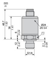
(1) SW24 tightening torque ≤ 25 N.m / 221 lb-in
