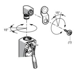
(1) Tightening torque (Min: 1) (Max: 1.5)
