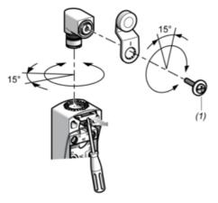
(1) Tightening torque (Min: 1) (Max: 1.5)
