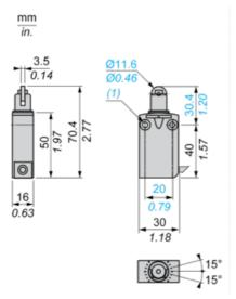
(1) 2 fixing holes  $\varnothing$  4.2 mm, counterbored  $\varnothing$  8 mm by 4 mm deep.
