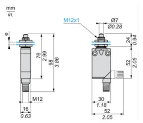
e : 8 mm max, panel cut-out  $\varnothing$  12.5 mm, fixing nut thickness 3.5 mm.
