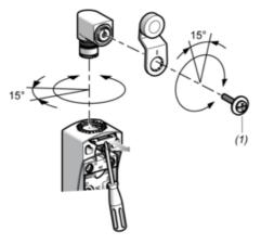
(1) Tightening torque (Min: 1) (Max: 1.5)
