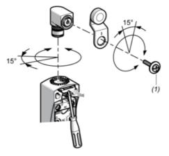
(1) Tightening torque (Min: 1) (Max: 1.5)
