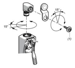
(1) Tightening torque (Min: 1) (Max: 1.5)
