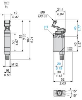
(1) 2 fixing holes Ø 4.2 mm, counterbored Ø 8 mm by 4 mm deep.
