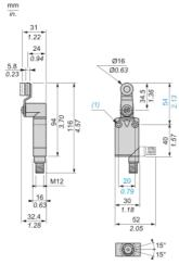
(1) 2 fixing holes  $\varnothing$  4.2 mm, counterbored  $\varnothing$  8 mm by 4 mm deep.
