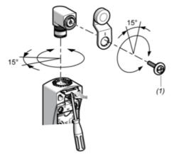
(1) Tightening torque (Min: 1) (Max: 1.5)
