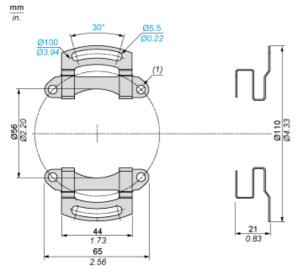
(1) 4 holes Ø 5.2 at 90° on 78 PCD. TH M5 x 6 screw fixings
